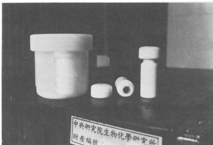
Fig. 1. PTFE vials and container shown inside a commercial microwave oven. The thicknesses of the two PTFE vials (right) and the container (left) are 6 and 5 mm, respectively. The container is 7.5 cm high with I.D. 7.5 cm and the vials are 5.5 cm high and with O.D. 3.0 and I.D. 1.8 cm. At the top of the small vial, a sealing septum of silicone-rubber was attached (not shown) for insertion of a needle to flush the vial with inert gas (e.g., nitrogen) before the microwave heating. The container can contain 1–5 vials at one time. It is preferably placed at the same location to ensure constant and reproducible heating.
